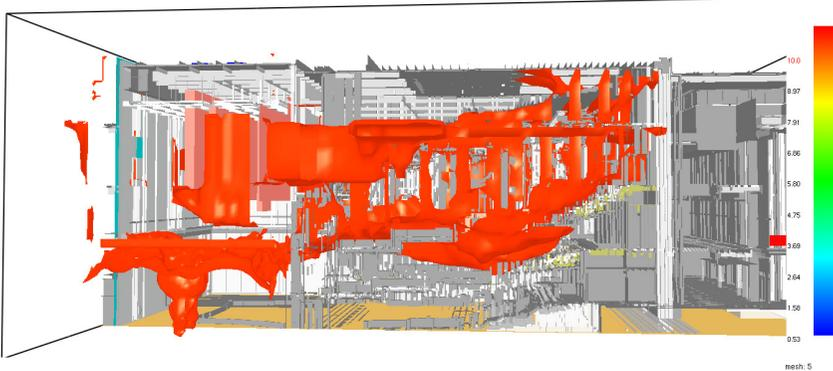
Fig. 4. 21,100 KW (20,000 Btu/s) Design Fire - Isosurface indicating smoke layer height (visibility at 10 meters) at 420 seconds.
