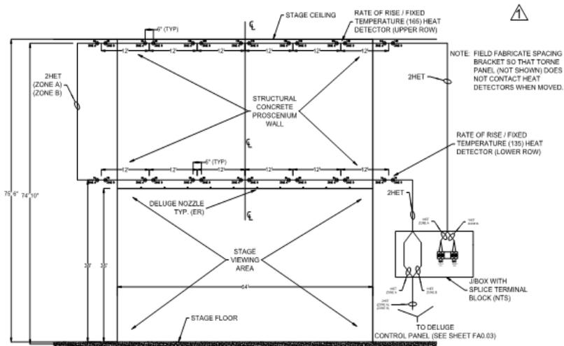
Fig. 1. Location of rate-of-rise and fixed temperature heat detectors.
