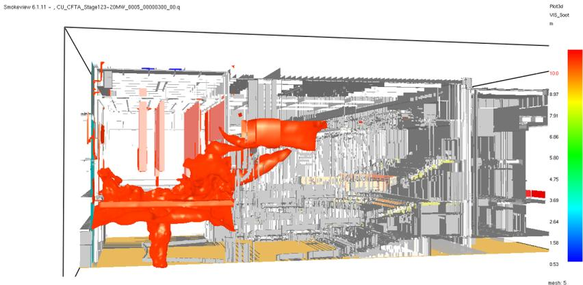
Fig. 2. 21,100 KW (20,000 Btu/s) Design Fire - Isosurface indicating smoke layer height (visibility at 10 meters) at 300 seconds.
