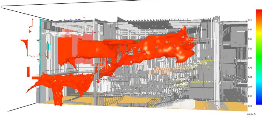
Fig. 3. 21,100 KW (20,000 Btu/s) Design Fire - Isosurface indicating smoke layer height (visibility at 10 meters) at 360 seconds.
