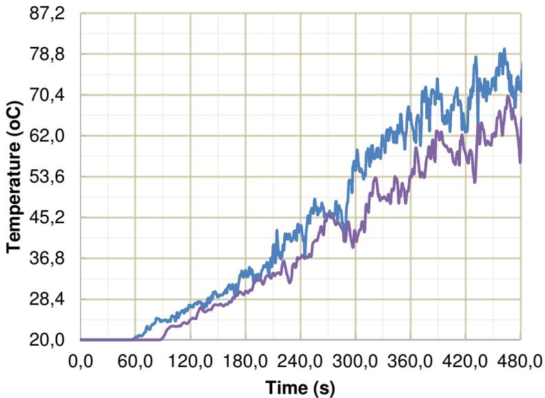
Fig. 5. Thermocouple measurement of heat detector temperatures at the top of stage.
