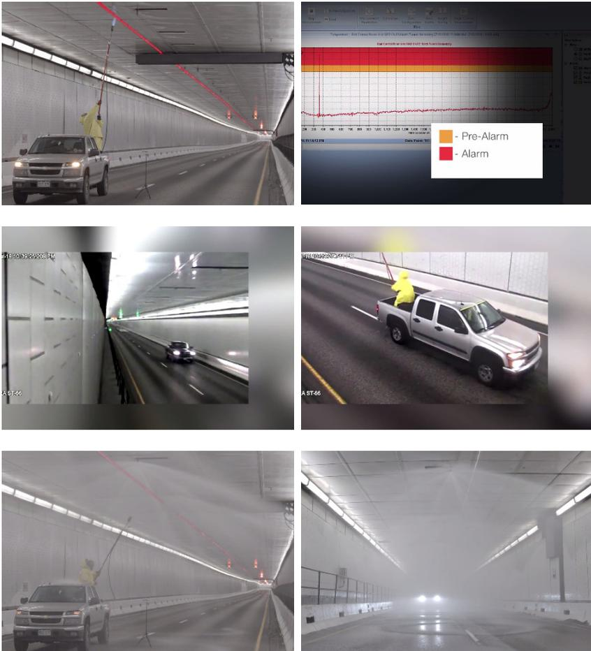
Fig. 4. Illustration of the system's operation during fire trial.
