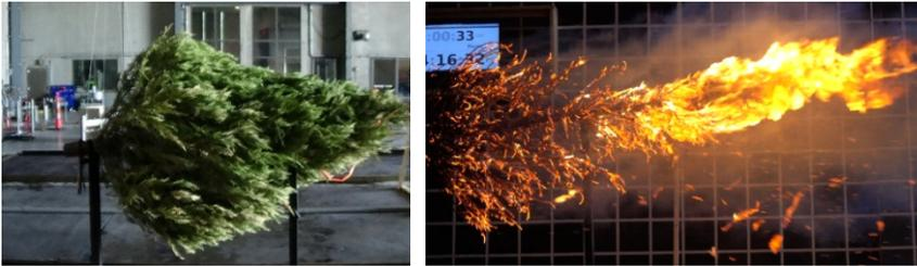
Fig. 1. (Left) A horizontally oriented tree before burning by a star-type gas burner from the left through the wind tunnel boundary layer, and (right) generated firebrands from the same burning tree.
