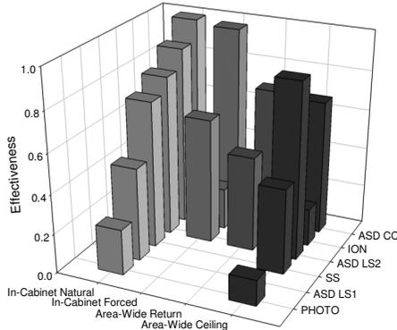
Fig. 5. Detector effectiveness in reaching ‘alert’ threshold during incipient stage by application.
