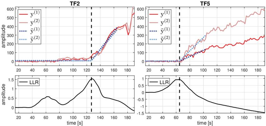
Fig. 2. Top: Examples of 2-channel signals ( $y^{(1)}, y^{(2)}$ ) recorded during two EN 54-7 test fires. Vertical lines indicate the event detection time. Estimated signals from the model fit at this time are ( $\tilde{y}^{(1)}, \tilde{y}^{(2)}$ ). Bottom: Computed LLR at each time step.
