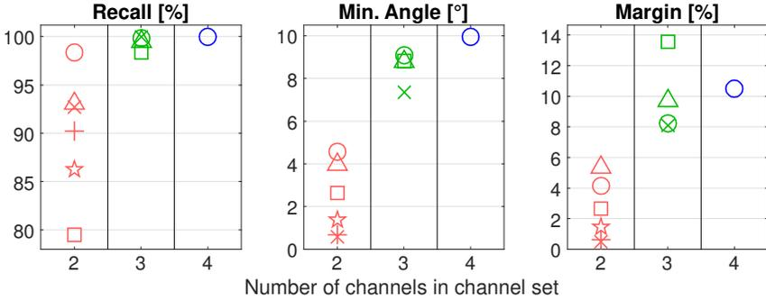
Fig. 5. Channel selection criteria for classification of fires vs. nuisances. For each number of channels, different symbols indicate different channel sets.
