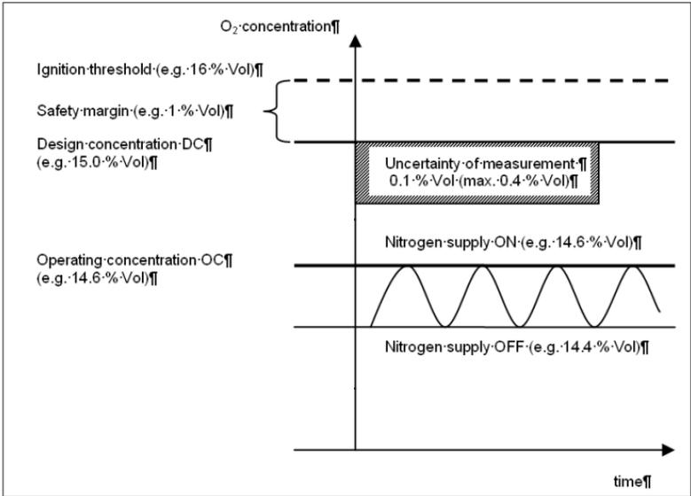
Fig. 1. Example of safety margins between ignition threshold and maximum operating concentration.
