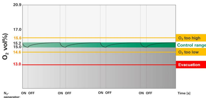
Fig. 2. Example of controlled oxygen level and monitoring of abnormal conditions.
