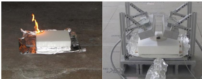
Figure 1. A flaming polyurethane foam slab ignited in a corner of the slab (left), and a smoldering polyurethane foam slab heated by radiant panels with a lit cigarette on a cotton fabric disk to initiate smoldering (right).
