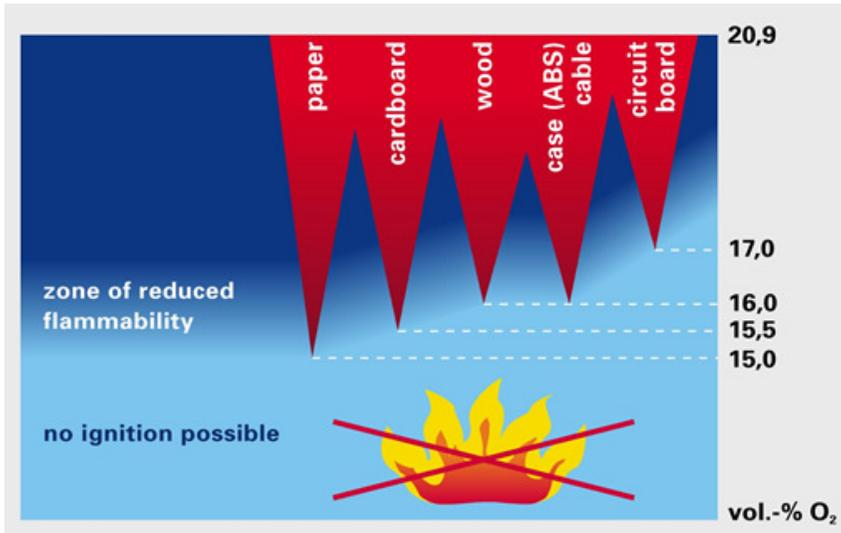
Fig. 2. Ignition limits for solid combustibles.
