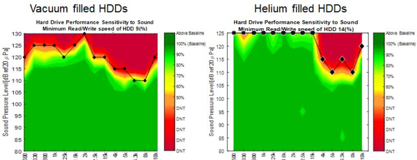
Figure 4. HDD sound characterization.
