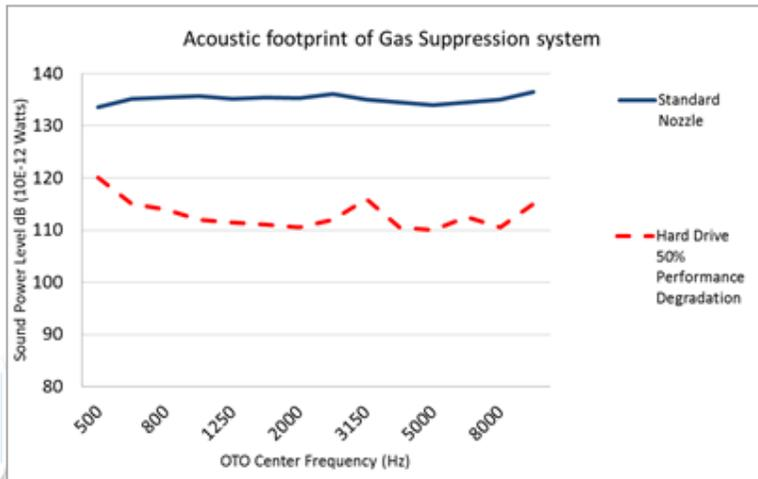
Figure 2. Inert gas fire protection system noise level comparison to HDD performance.
