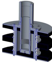
Figure 5. Standard Inert Gas Nozzle.      Figure 6. Acoustic Nozzle X-Section.
