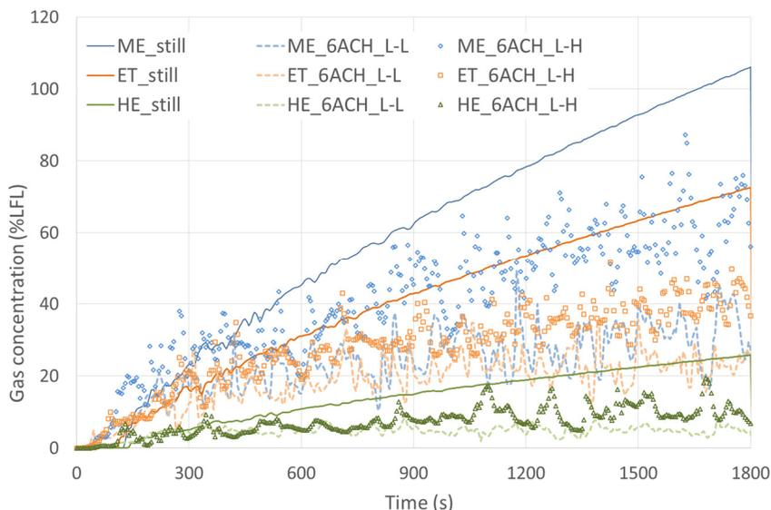
Figure 3. Maximum gas concentrations from 25 m<sup>2</sup> pool evaporation.
