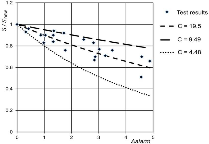
Fig. 2. Results of tunnel tests on smoke chamber after contamination with dust.
