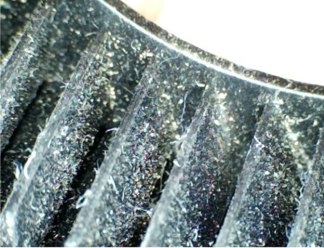
Fig. 1. Dust on surface of smoke sensing chamber at a  $\Delta_{alarm}$  of 4.4.
