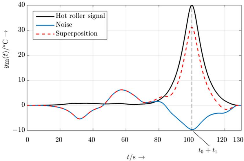
Fig. 12. Output signals for the matched filter: Contributions of the hot roller, the noise, and superposition of hot roller and noise.
