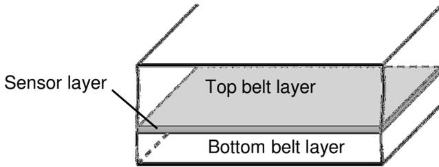
Fig. 5. Model for the heat transfer in a rubber belt with integrated sensor element: Top and bottom layers: rubber, central layer: temperature sensor.
