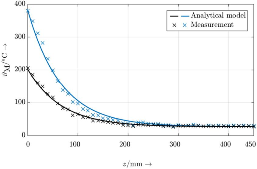
Fig. 4. Temperature on a roller with overheated bearing as a function of axial position.
