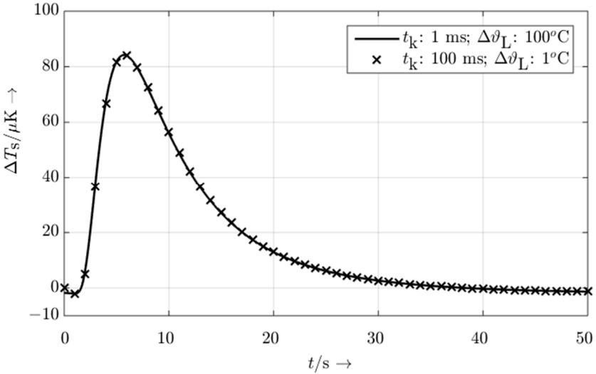
Fig. 9. Simulated sensor system's output signal for different input signals of overheated rollers.
