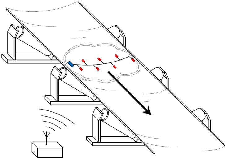
Fig. 1. Roller temperature monitoring system.
