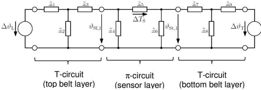
Fig. 7. Electrical equivalent circuit of the belt with implemented sensor system.
