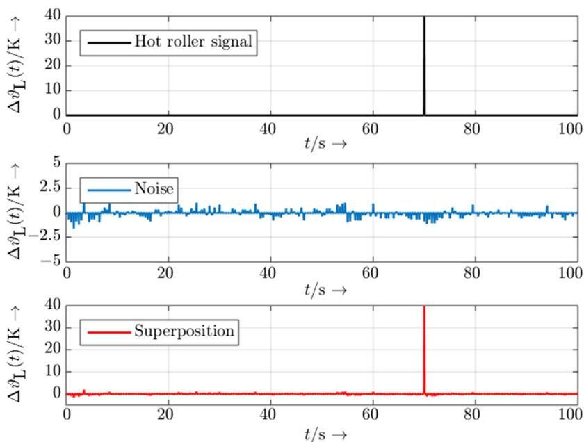
Fig. 11. Input signals for the matched filter. Top: Hot roller signal, middle: noise, bottom: superposition of hot roller signal and noise.
