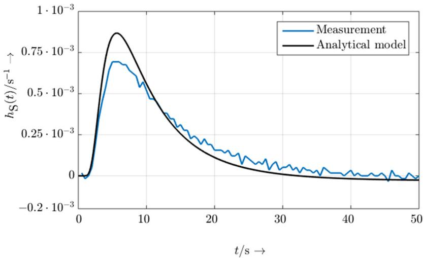
Fig. 8. Measured and analytically calculated impulse response.
