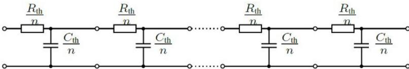
Fig. 6. Electrical equivalent circuit of each belt layer.
