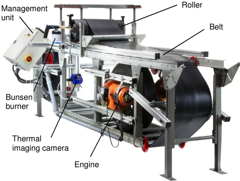
Fig. 3. Test mockup of a belt conveyor system.
