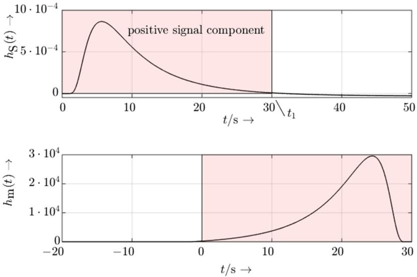
Fig. 10. Impulse responses of the sensor system  $h_S(t)$  and the matched filter  $h_m(t)$ .
