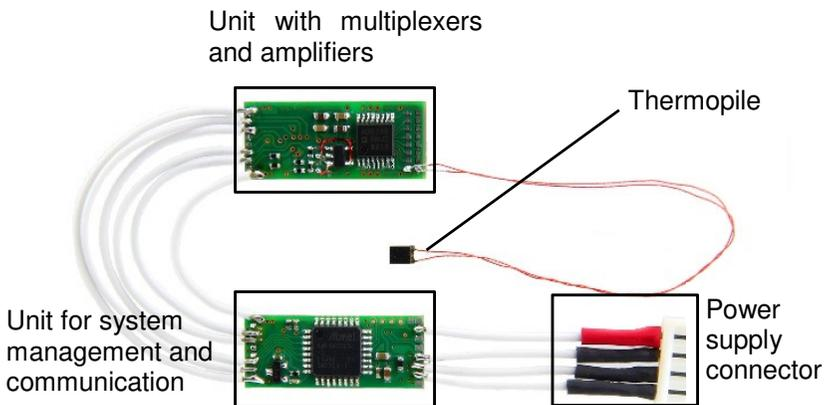
Fig. 2. Laboratory prototype of the sensor system.
