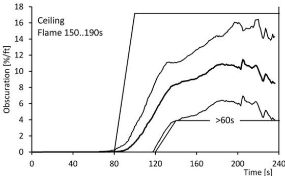
Fig. 1. Wood fire obscuration at ceiling and corresponding boundaries.
