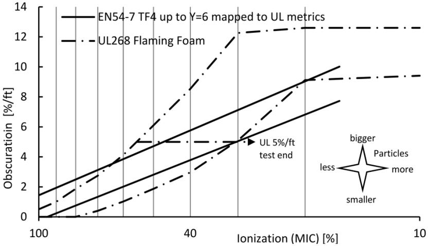
Fig. 10. Flaming polyurethane foam compare between UL and EN54.
