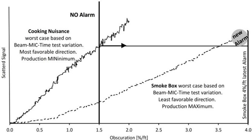
Fig. 8. Obscuration vs. forward scattered signal for cooking nuisance hamburger and smoke box sensitivity with cotton wick.
