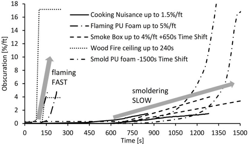
Fig. 12. Obscuration compare between fast flaming fires and slow smoldering fires resp. smoke box and cooking nuisance hamburger.
