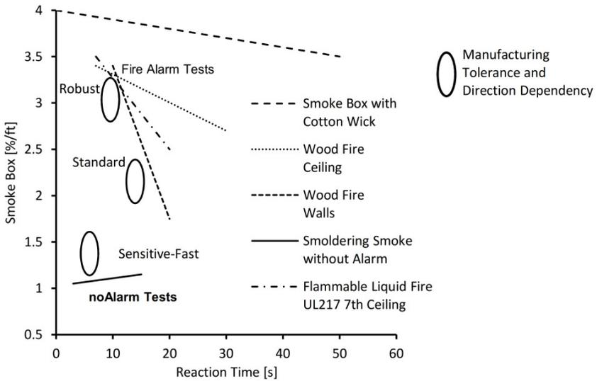
Fig. 4. Alarm regression diagram based on UL268 6th edition.
