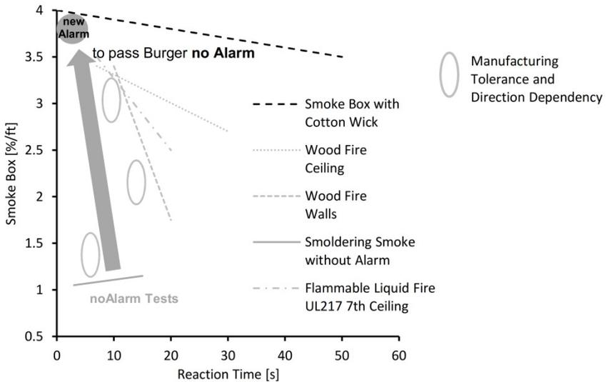
Fig. 9. Alarm regression diagram with added new cooking nuisance.
