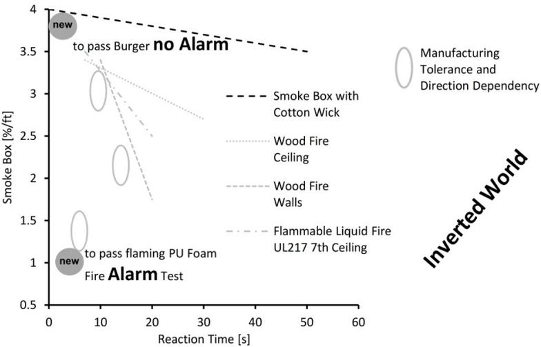
Fig. 11. Alarm regression diagram with cooking nuisance hamburger and flaming polyurethane.
