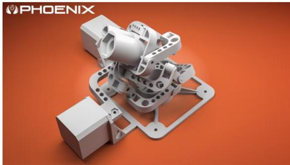
**Figure 3. Targeting Gimbal:** the target gimbal allows the IR sensor to be scan the environment and positions the extinguishing nozzle.
