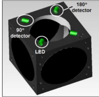
Figure 2. Model of the smoke detector chamber geometry.
