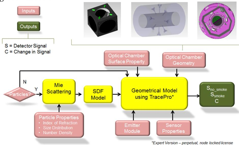
Figure 1. Model Architecture that incorporates Mie scattering, the scattering distribution function (SDF) and ray tracing approaches for a physics based assessment of multi-wavelength smoke detection systems.
